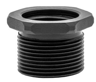
MANUFACTURED: USA MATERIAL: 4140HT STEEL FINISH: BLACK NITRIDE OR STAINLESS STEEL SIZES: 1/2-28 TO 5/8-24 9/16-24 TO 5/8-24
